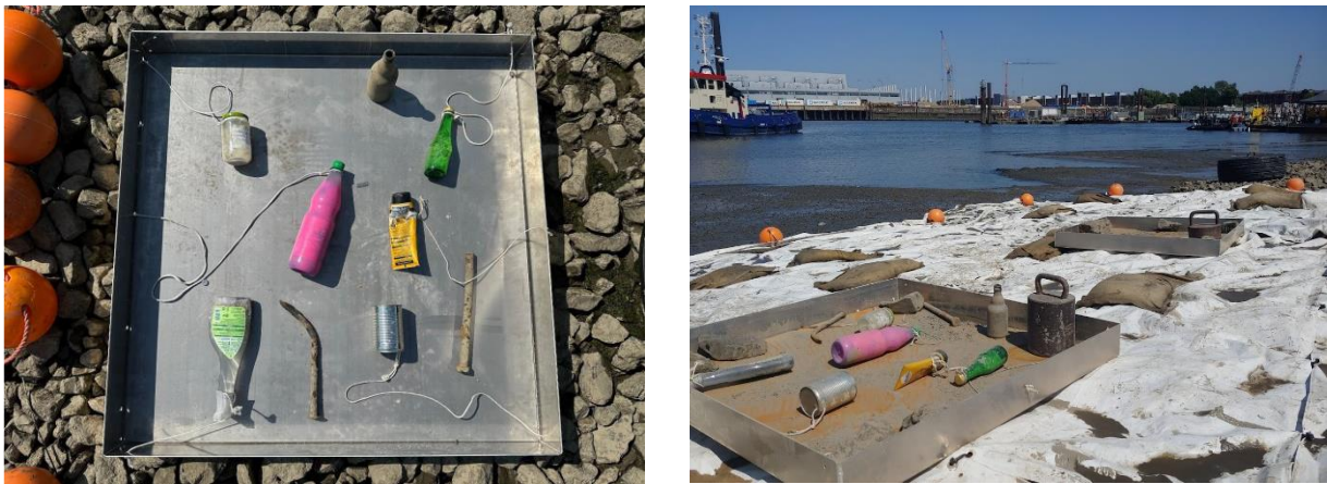
Figure 4: Litter trays from sheet metal with samples tied to them and placed on the seabed during low tide.
